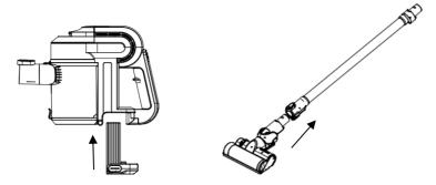
**Step 2:** Install the electrical brush by inserting it into tube carefully.
